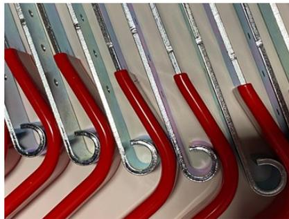
In 2018, the shop added dip coating lines, which enables it to add a thick, protective coating to parts that have an unusual shape, such as football facemasks.
